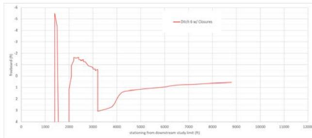
Figure 3.3-16. Estimated freeboard along Ditch 6 for the planned left levee.
