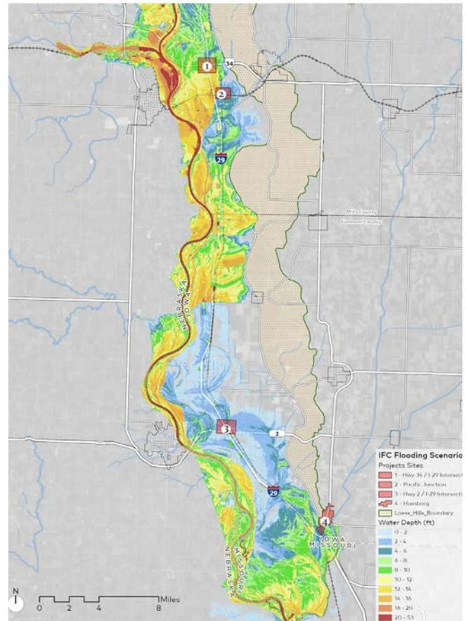
Figure 0-2. Flooding inundation modeling, 2019 Flood (Iowa Flood Center).
