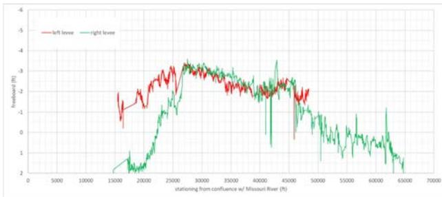
Figure 3.3-12. Estimated freeboard along the Nishnabotna River for the left and right levees.
