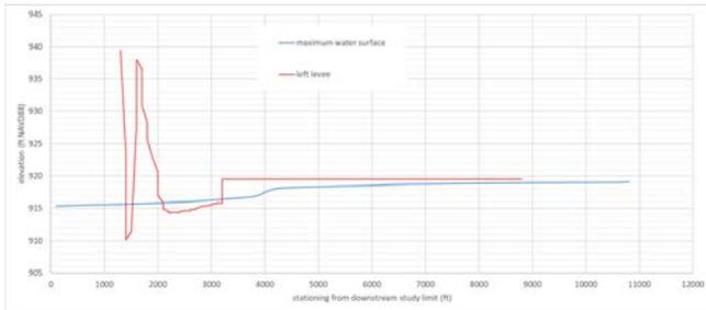
Figure 3.3-15. Water surface elevation profile along Ditch 6, also including Missouri River water surface elevations under natural valley conditions, shown with left top of levee elevations.
