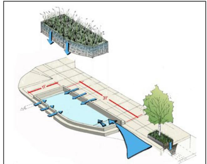
Diagram of how a stormwater bumpout works
