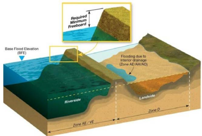
Figure 3.2-7. Cross section of a reach modeled using Sound Levee Procedure.
