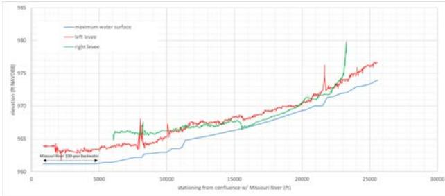
Figure 3.3-20. Water surface elevation profile of the Keg Creek shown with left and right top of levee elevations.
