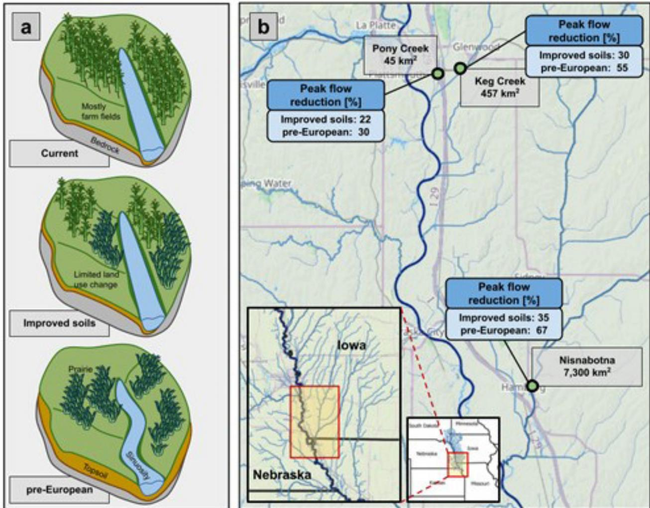
Figure 3.3-6. (a) Model setups - Current (Scenario G), Improved soils, and Pre-European. (b) Gauging sites and percentage peak flow reductions relative to the Current conditions scenario.
