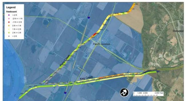
Figure 3.3-19. Depiction of inundation behind the levees if Pony Creek is overtopped at lowest freeboard location.
