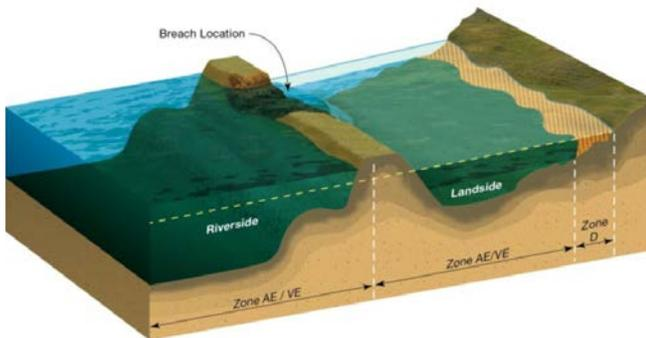
Figure 3.2-4. Cross section of a reach modeled using Structural Based Inundation Procedure.
