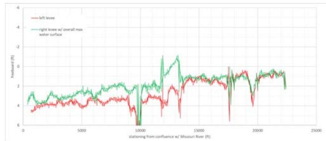
Figure 3.3-23. Estimated freeboard along Pony Creek for the left and right levees.
