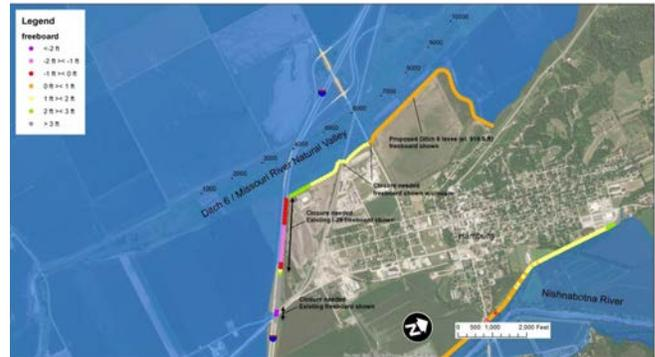
Figure 3.3-13. Estimated freeboard along Ditch 6 near Hamburg, Iowa. No overtopping allowed.
