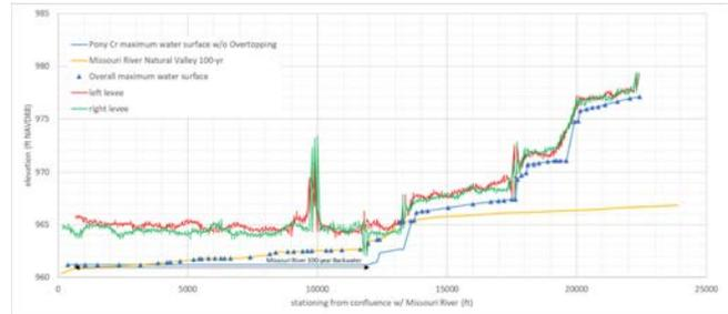
Figure 3.3-22. Water surface elevation profile of Pony Creek and Missouri River water surface elevations under natural valley conditions shown with left and right top of levee elevations.
