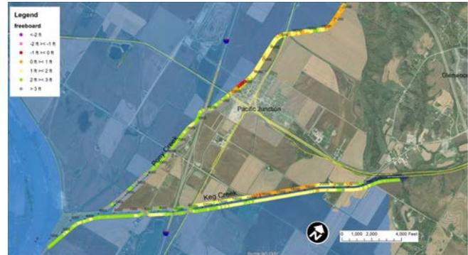
Figure 1.0-5. Freeboard/levee analysis at Pacific Junction. Levees.
