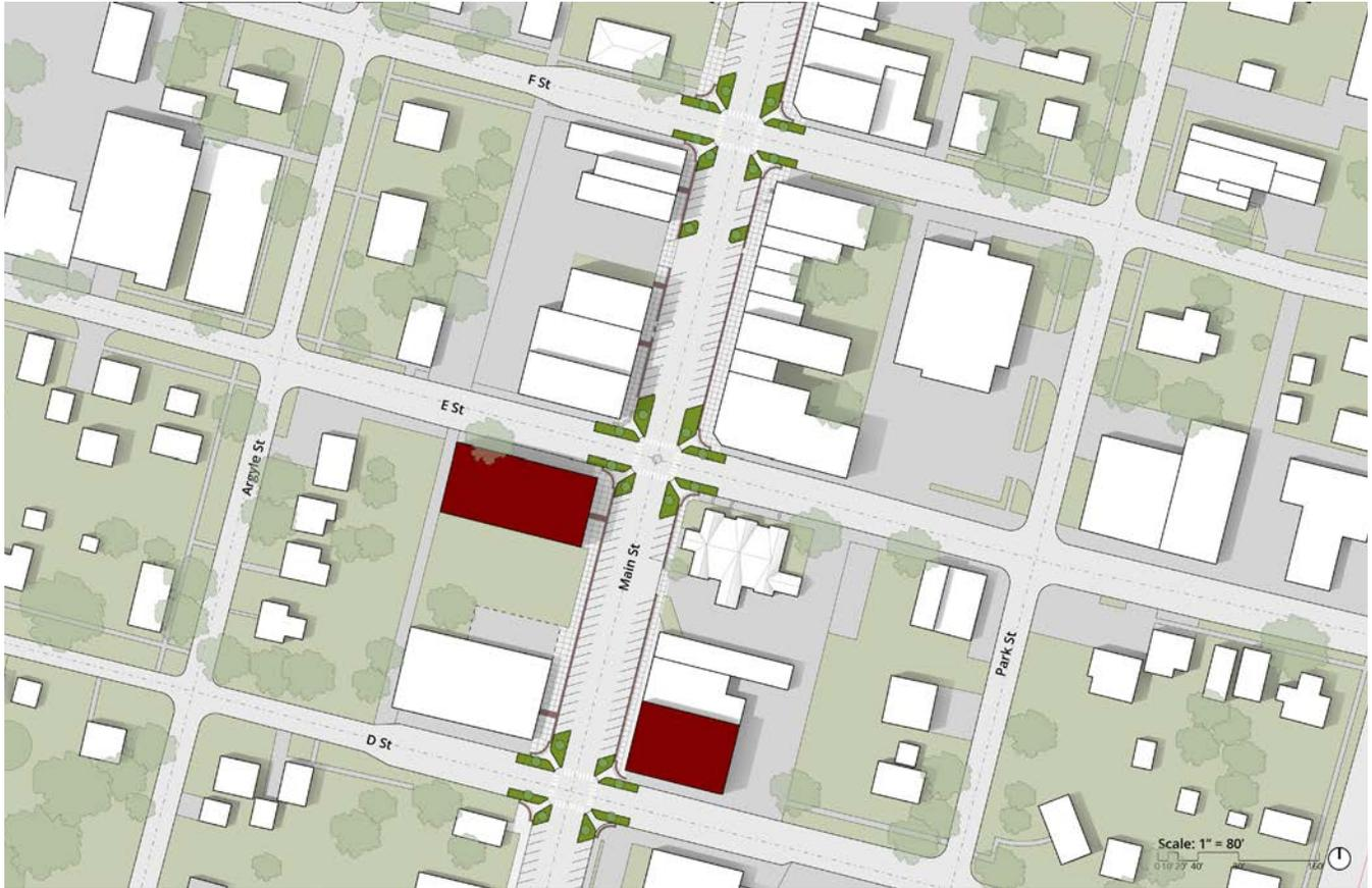
Site plan for Main Street stormwater bumpouts
