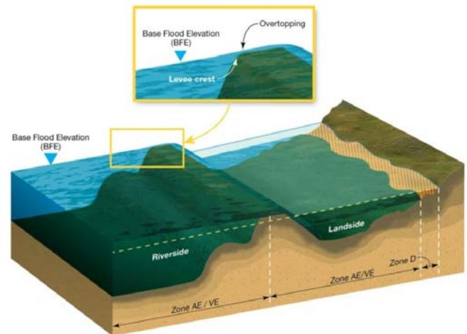
Figure 3.2-5. Cross section of a reach modeled using Overtopping Procedure.
