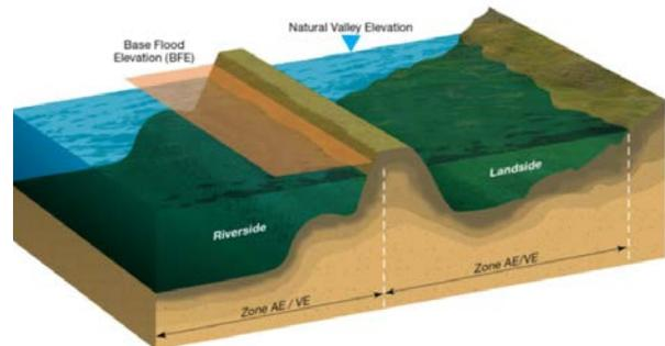
Figure 3.2-3. Cross section of a reach modeled using Natural Valley Procedure.
