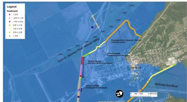
Figure 3.3-14. Depiction of inundation behind the levee if the I-29 closure structure is not in place.
