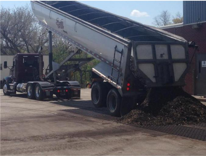
**Truck Delivering Coal and Woodchip Mixture**
